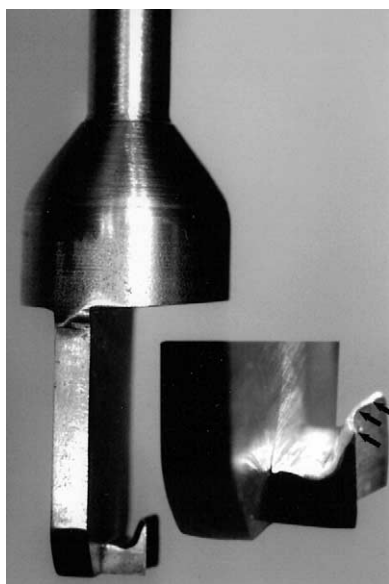
Fig 1. Custom shearing rod (Bulut-type shearing blade) of testing apparatus. Contour of edge (arrows) matches contour of bracket base (see Fig 2).
